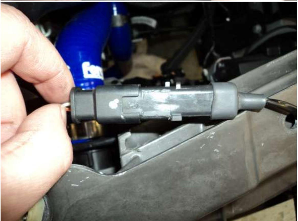
5. Plug one end into the connector that was taken off of the standard valve and plug the other end into the solenoid. Once done use the cable ties provided to secure the loom.
