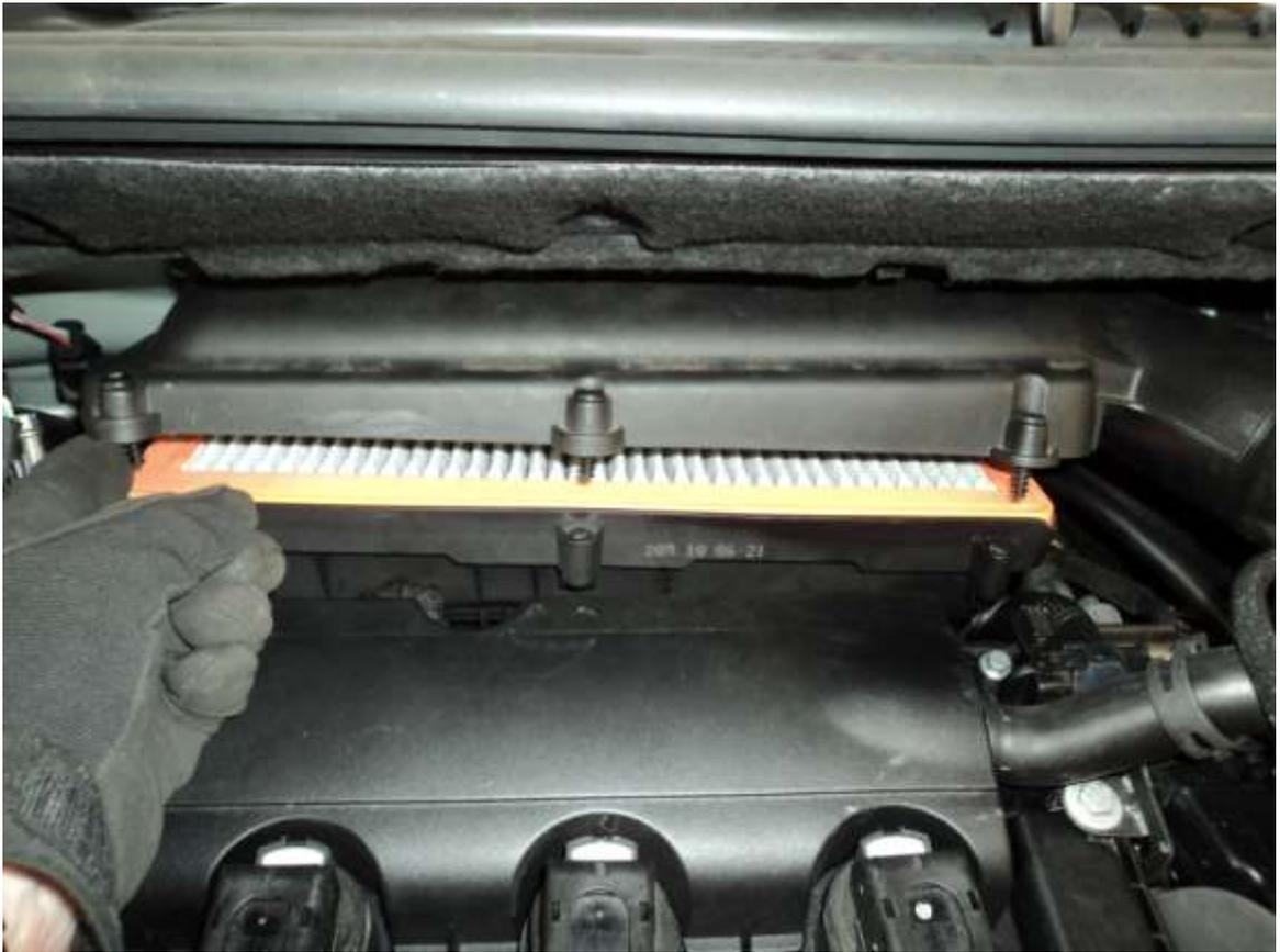
8. Remove the bottom of the air box by pulling upwards to release it from its rubber mounts.
