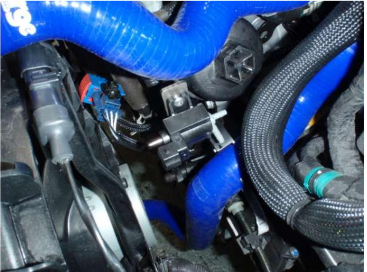
4. Use the wiring loom provided. You will need to trim the 2 small lugs on one end to make it fit into the oem plug.
