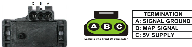
Figure 5 – Manifold Absolute Pressure Sensor and harness Termination
