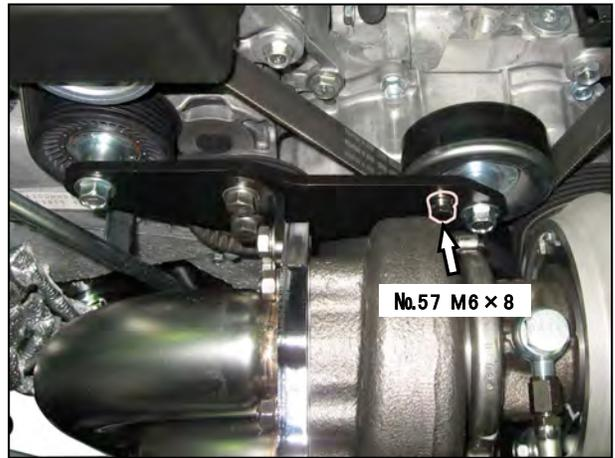
(2) Install the Turbine Heat Shield by sliding the cut outs over the down pipe hardware as shown in the photo.
