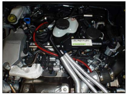
6. At the back of the engine on the inlet manifold next to the throttle body unclip the rubber pipe. Using the silicon hose and coupler supplied in the kit attach as shown and connect to the vacuum hose.
