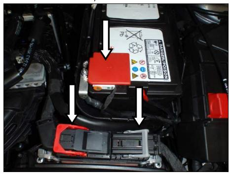
2. Unclip the ECU remove air filter cover and the filter, remove the plastic clips on the cold air scoop and undo the jubilee clips on both ends of the flexible intake hose. Now remove the scoop and filter box undo the bolt attaching the flexible hose and pipes. Rotate the flexible hose and pipes so access to the BOV blanking plate can be removed.
