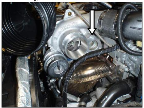
4. Bolt on the BOV with the vacuum port in the position shown below with the vacuum hose going behind the turbo outlet.
