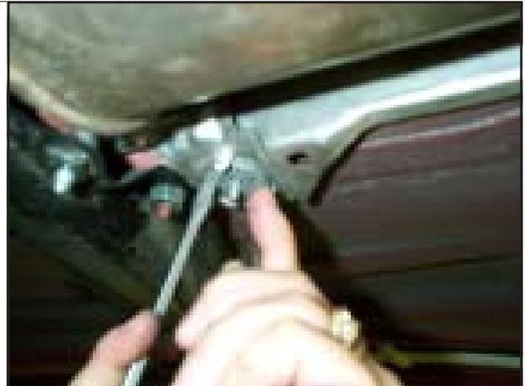
**STEP 3.** Loosen exhaust coupling bolts.
