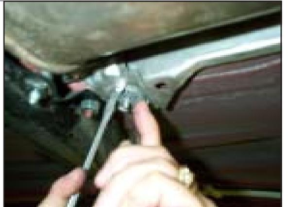
**STEP 51.** Reinstall center exhaust support.
