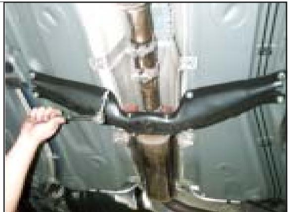
**STEP 7.** Remove center heat shield.
