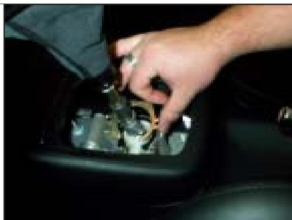
**STEP 19.** Pull stick upward and remove pivot bushing.
