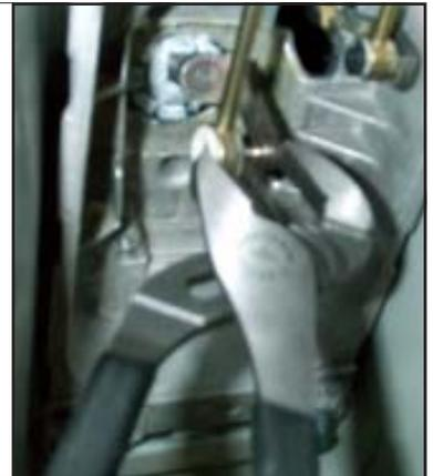
**STEP 46.** Reinstall retaining ring onto shifter.
