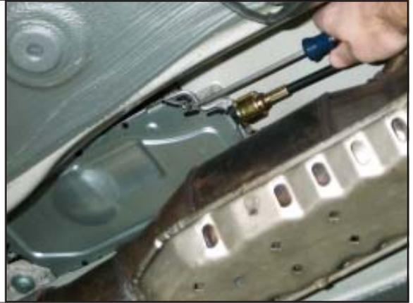
**STEP 9.** Remove retaining clip from shifter.
