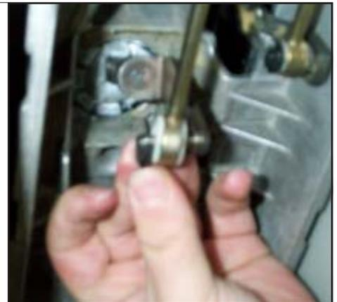
**STEP 47.** Reinstall bottom plate on shifter enclosure.
