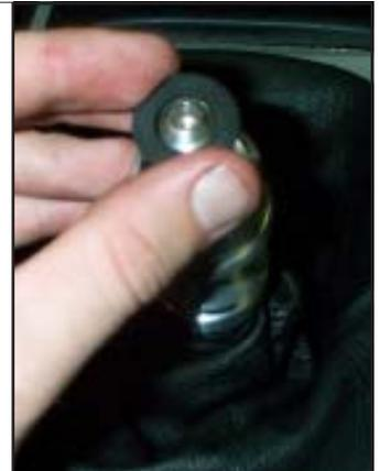
**STEP 38.** Install reverse lockout spring.
