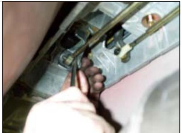
**STEP 11.** Remove retaining clip from shift linkage.
