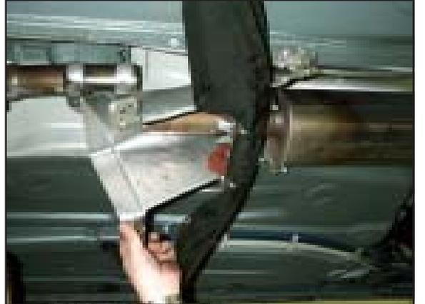
**STEP 50.** Reinstall heat shield snap washers.
