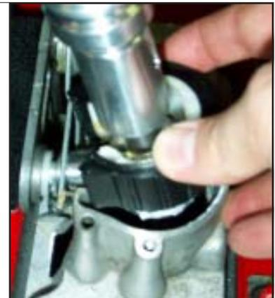
**STEP 27.** Fully seat **B&M Short Throw Shifter** assembly into base.
