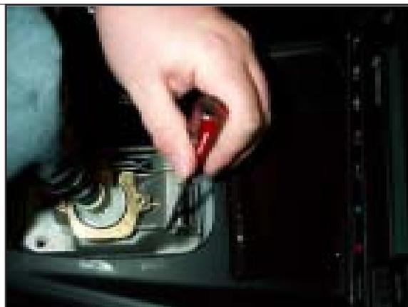
**STEP 17.** Remove bolts securing top plate.
