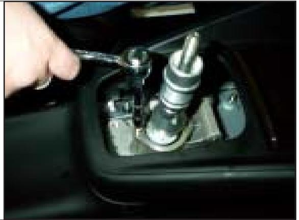
**STEP 32.** Install retaining clip removed in step 16.
